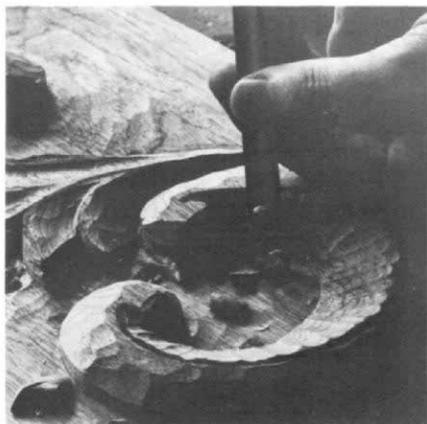
*A quick gouge rough-shapes the wood on the inside curves.*
