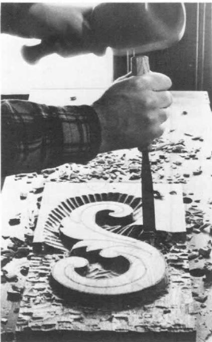
*Remove background waste with closely spaced vertical cuts.*
