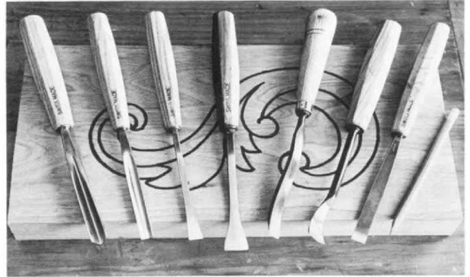
*Relief carving tools (from left): V-tool for outlining, three gouges for general shaping, long bent grouter for backgrounds, spoon gouge, and flat or firmer gouge. The blank is butternut, held to the bench by a long screw from underneath.*
