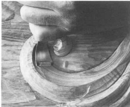
*Long sweep cuts leave a smooth finish. A bent gouge or spoon gouge may be best for inside curves. The right hand powers the tool, while the edge of the left hand rests firmly on the work.*
